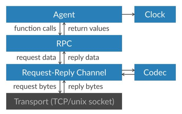
1. The channel layer allows you to send and receive actual data like strings, lists ob numbers instead of single bytes.
